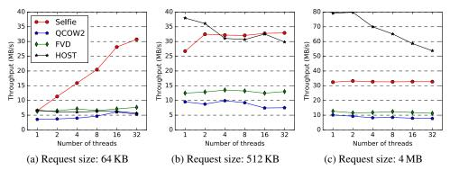
Figure 5: Throughput of fio with the virtual image hosed on the logical volume and each thread making sequential accesses.
