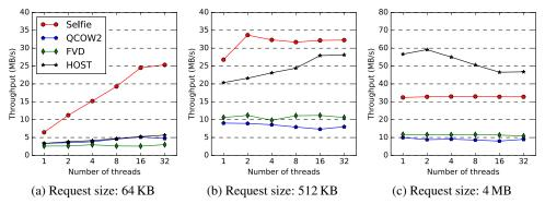
Figure 6: Throughput of fio with the virtual image hosed on the logical volume and each thread making random accesses.
