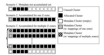
Figure 4: Accumulating mapping info into metadata clusters.
